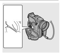
it up, releasing and lifting it out. Make sure to attach a power source to the camcorder first, so it will retain your chosen settings when you change the battery.
